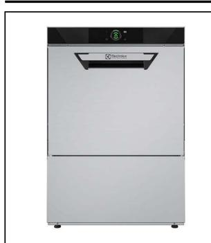
400301 (ETUCLIS) Undercounter Dishwasher (L), touch control, single skin with pressure boiler, rinse aid pump, max. 65 r/h, 1 phase, Schuko plug
